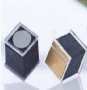
3D Image Sensor Module (RGB front camera, IR Projector, IR stereo Camera)
